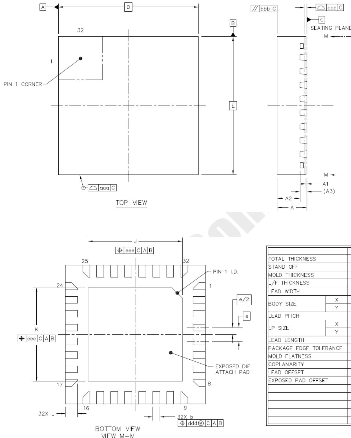
Figure 11: QFN 4 x 4 mm Package Dimensions
