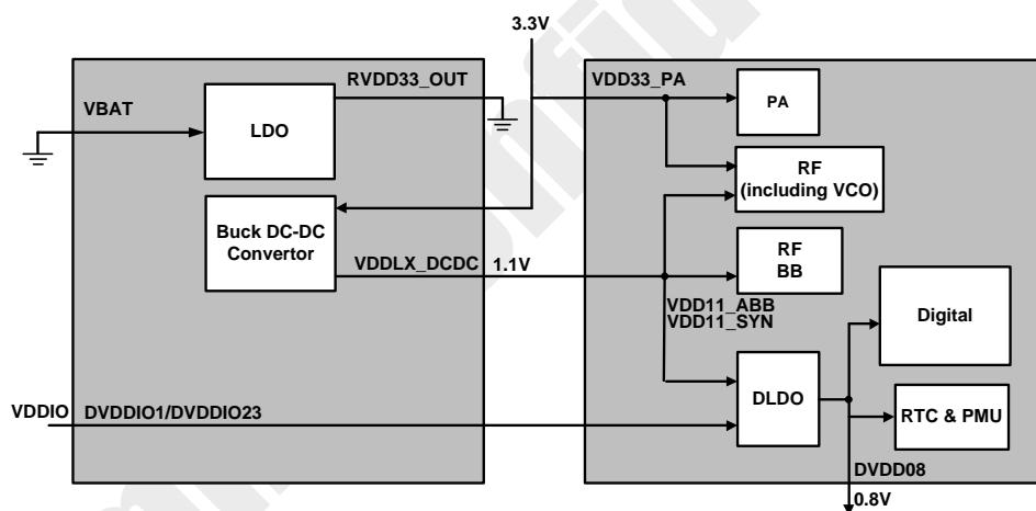
Figure 2: SV6158-M typical Power Connection
