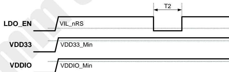
Figure 5: Reset Timing with typical power
