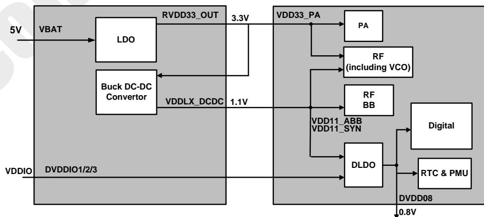
Figure 3: SV6158-M Power Connection with Internal LDO
