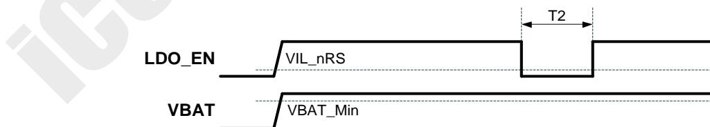
Figure 7: Reset Timing with Internal LDO
