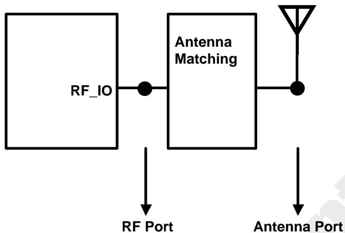
Figure 9: RF Front-End Reference Topology for RF Performance
